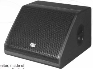
The MR15C is a high precision and high power stage monitor, made of high quality plywood with polyurea paint. It offers a "studio monitoring" type of response, exceptional dynamic capability and very low distortion. Fitted with one 15" woofer and one 1" exit neodymium compression driver coupled to a patent 90° x 40° horn. MR15CA is equipped with FA1.6 digital amplifier module based on MR15C to be an active monitor.
