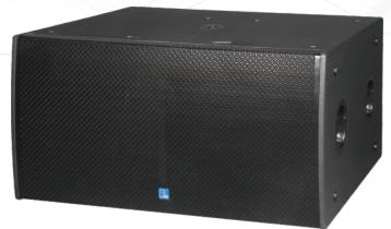
**DLA221B** is a dual 21" subwoofer. It features 2x21" 115mm voice coil woofer, bass-reflex design, can be used with line array and point source full range speakers to improve the low frequency performance. The cabinet is made of multilayer composite plywood with wear-resistant polyurea paint.
